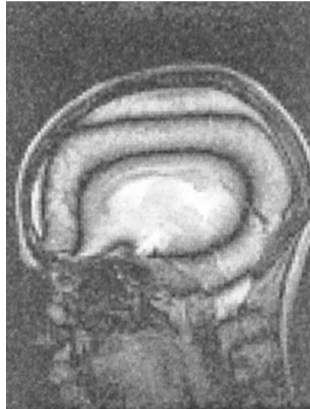
Figure 2.11. B_1 fringes with ‘one pulse M_z ’ scheme C. A hard 1800^\circ pulse followed by two-dimensional gradient echo readout gives B_1 fringes. Light and dark rings occur at intervals of 5% change in B_1 . Dark rings occur at intervals of 10%. For other values of hard pulse FA, the interval is (1800^\circ/\text{FA})\% . Reprinted with permission from Deichmann, R., Good, C. D. and Turnes, R. 2002, RF inhomogeneity compensation in structural brain imaging, in Magn. Reson. Med. , Copyright 2002 John Wiley & Sons Inc.
